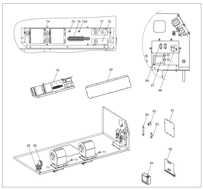
Figure 26. Electrical Components.
